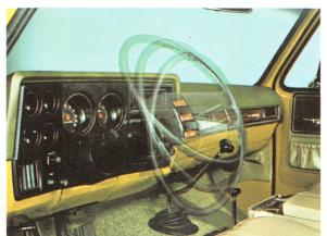
Six-position tilt steering is available with Turbo Hydra-Matic or four speed manual transmissions. Adjustable for driver preference and comfort.
